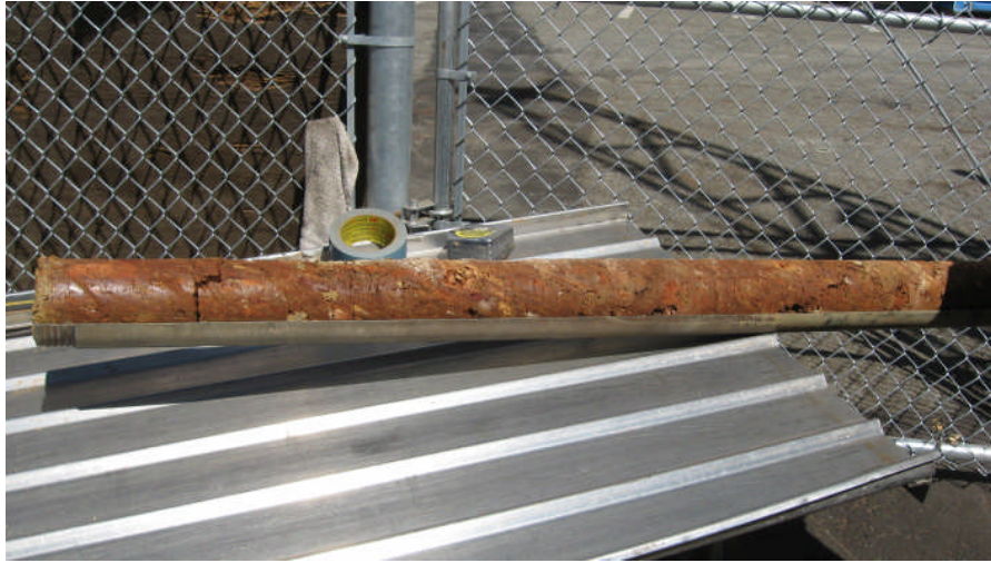
Photograph 5: View of exposed soil core sample after removal from casing, facing east
